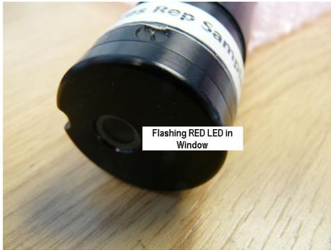
Whilst the **red** led on the VMT is flashing once per second, remove the magnet from the side of the VMT.
