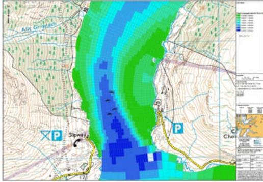
Figure 10 Map of the rates of flow at peak flood tide in the Kylerhea study site with the approximate locations of the four proposed tidal turbines indicated by the black symbols and current speed indicated by colour, with green representing low flow rates and blue representing higher rates. (reproduced from MCT.)
