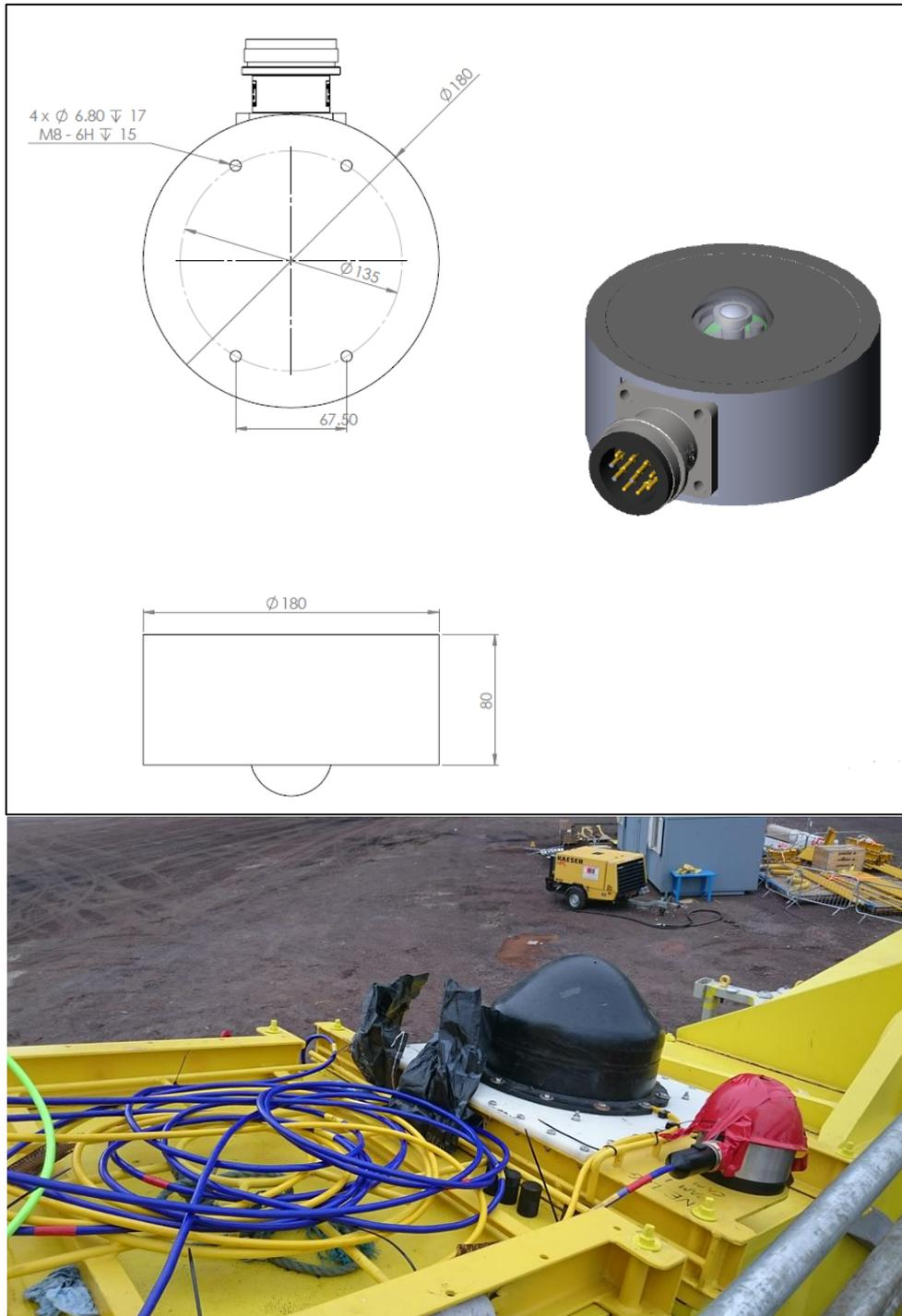
Figure 3. Schematic of the video camera (upper) and a photograph of the PAM module and video camera (lower) mounted on Atlantis AR1500 TSS (under a hard hat to protect the lens during construction).
