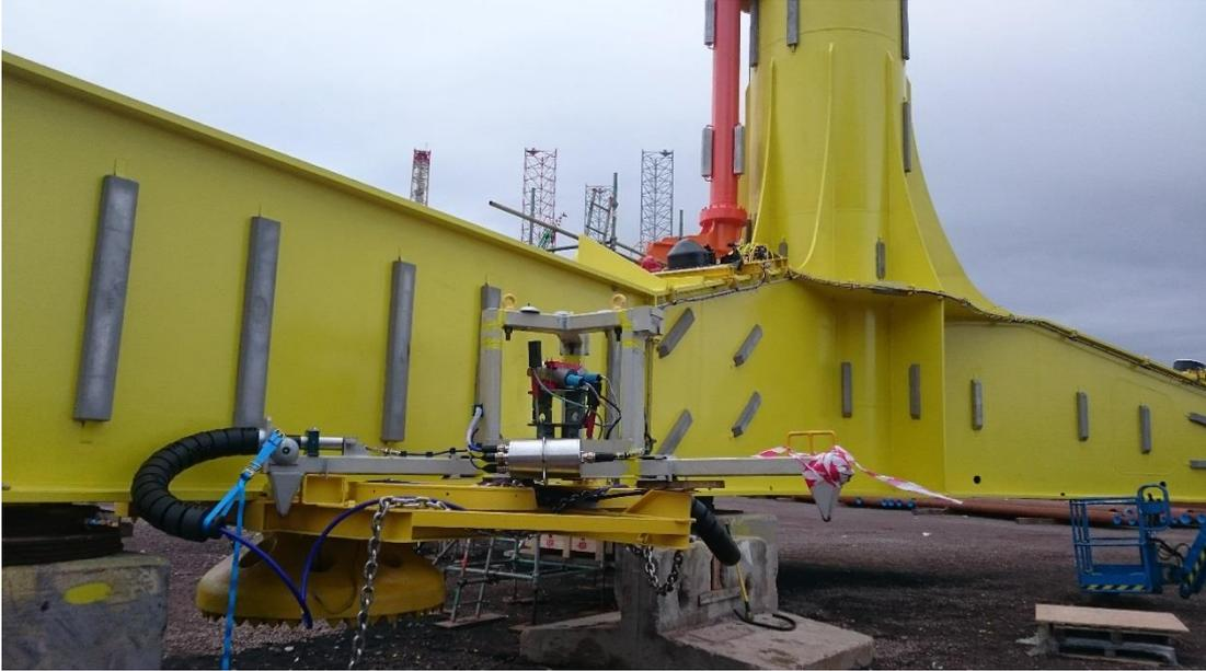
Figure 5. HiCUP mounted on the Atlantis TSS assembly prior to load out and deployment in the Inner Sound.
