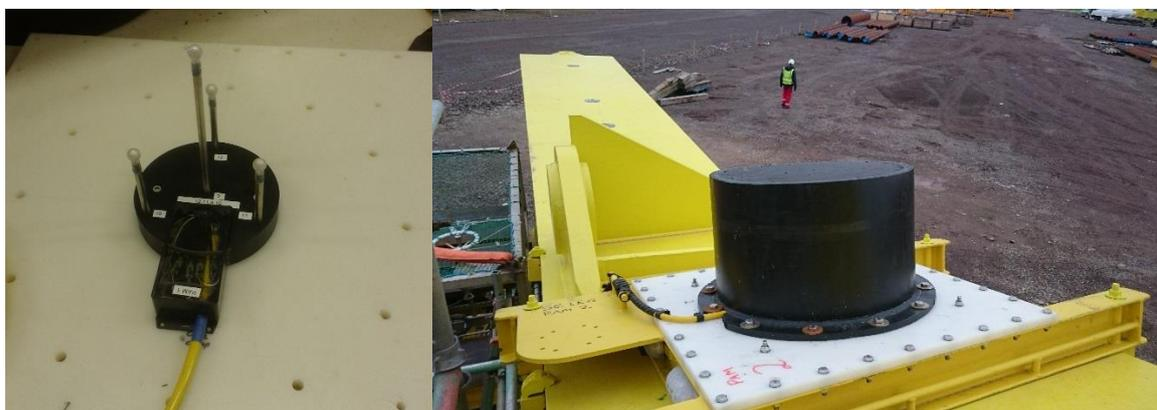
Figure 1. PAM four channel tetrahedral cluster during assembly (left) and mounted within its housing on the Atlantis TSS leg (right).
